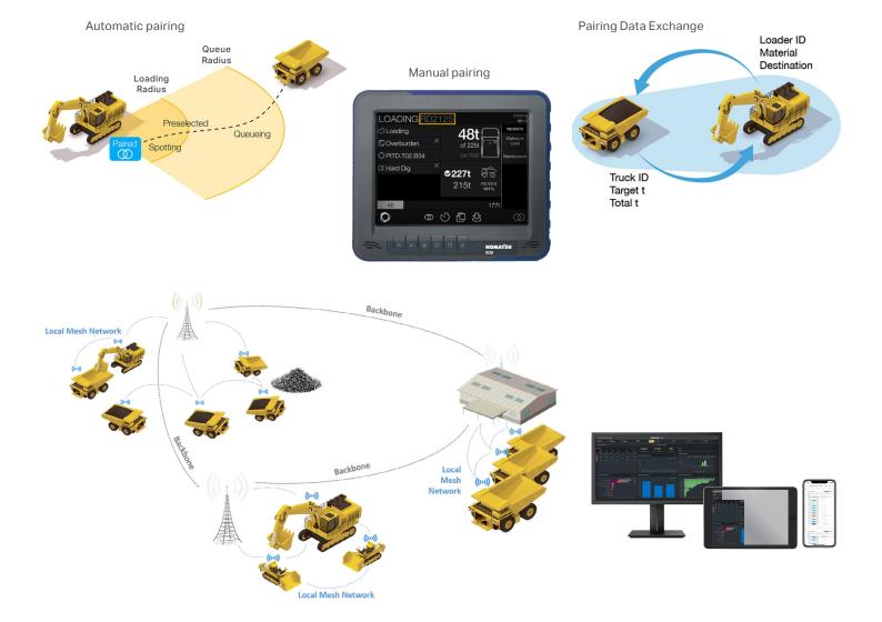
The Komatsu iSite Mesh Network is made up of a collection of wireless networking devices running Komatsu iSite mesh networking software.
