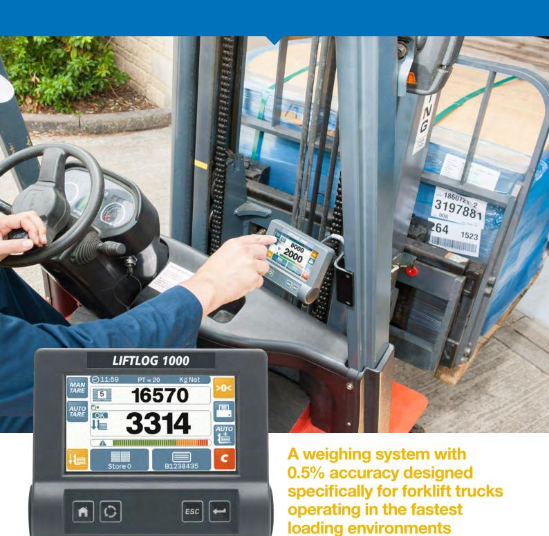
With the ever increasing focus on productivity and safe-loading, the new *LIFTLOG 1000* is a cost-effective weighing instrument that reduces loading cycle times and maximises tons per hour performance.
