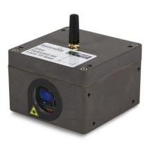
The FlatMesh Optical Displacement Sensor Node is an instrument which uses optical means to take high precision displacement measurements and pass these through Senceive's FlatMesh wireless communications network to a FlatMesh Gateway. It can also be combined with Senceive's world-leading triaxial tilt sensor to obtain high precision tilt measurements that are linked to an external reference.
