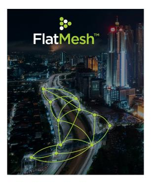
In a FlatMesh™ system the devices 'talk' to their neighbours, relaying data in a series of hops to the outside world. This dynamic, non-hierarchical system is extremely robust and can tolerate damage to individual devices without systematic loss of performance. It is suited to dense networks concentrated in relatively small areas. It is particularly appropriate for sites that are difficult to access, with obstructions that would constrain other technologies.
