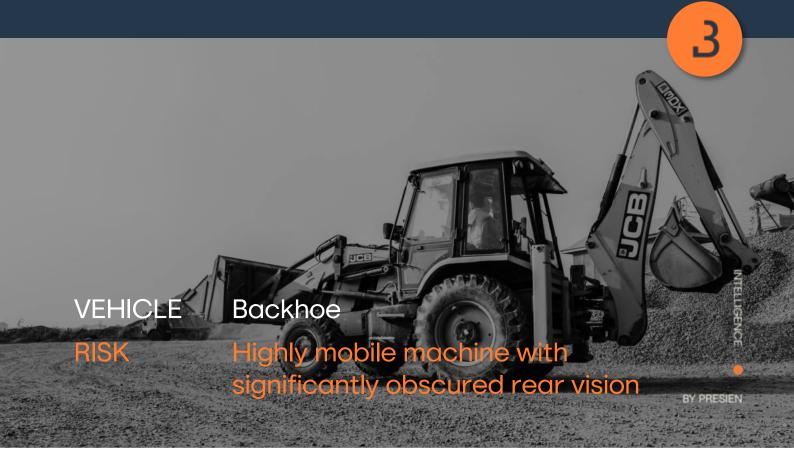
Operators and site health and safety were concerned of potential plant-people interaction at the backhoe's rear blind spot due to the quick and varied forwards and backwards operation of the vehicle.
