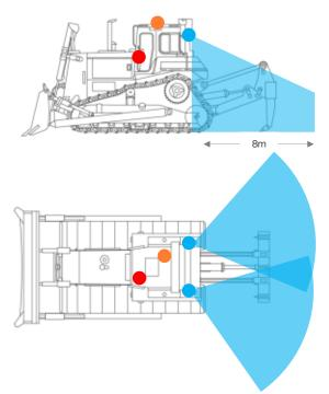
Hardware 1x Blindsight Processing Unit (BPU), 2x sensor with bolt mounts, 2x 5m cables, 1x incab alert.
