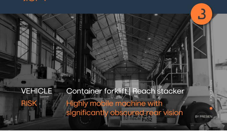
Operators and site health and safety were concerned of potential plant-people interaction at the forklift's rear blind spot due to the quick and varied forwards and backwards operation of the vehicle.
