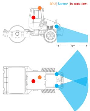
Hardware 1x Blindsight Processing Unit (BPU), 2x Sensor with bolt mount, 2x 5m cable, 1x Incab alert.
