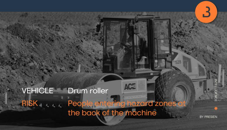
Operators and site health and safety were concerned of potential plant-people and plantplant interaction at the roller's rear blind spot due to the quick and varied forwards and backwards operation of the vehicle.
