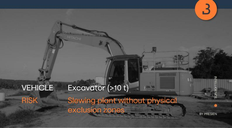
Operators and site health and safety were concerned about people entering the exclusion zone around the excavator. The machine completely obscures the operator's vision in the rear and right side, creating a dangerous potential for people-plant interaction.
