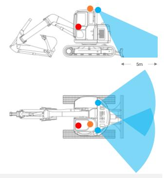
Hardware 1x Blindsight Processing Unit (BPU), 2x Sensor with bolt mount, 2x 3m cable, 1x In-
