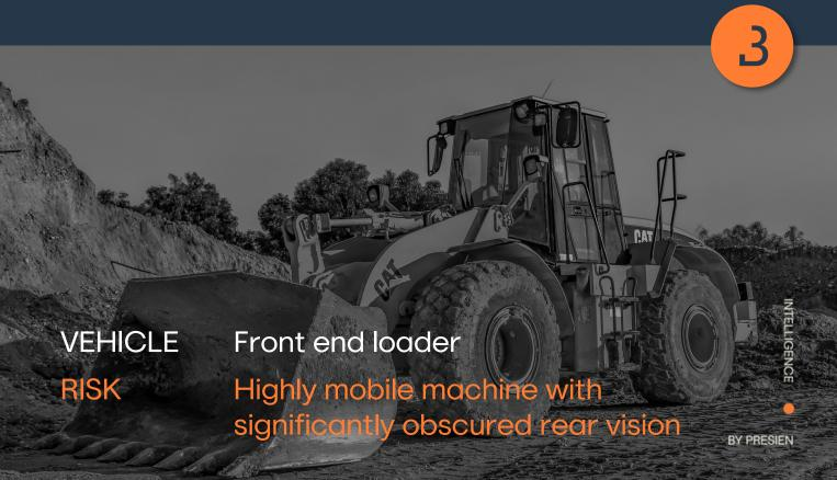
Operators and site health and safety were concerned of potential plant-people and plantplant interaction at the loader's rear blind spot due to the quick and varied forwards and backwards operation of the vehicle.
