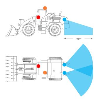
Hardware 1x Blindsight Processing Unit (BPU), 2x Sensor with bolt mount, 2x 5m cable, 1x Incab alert.
