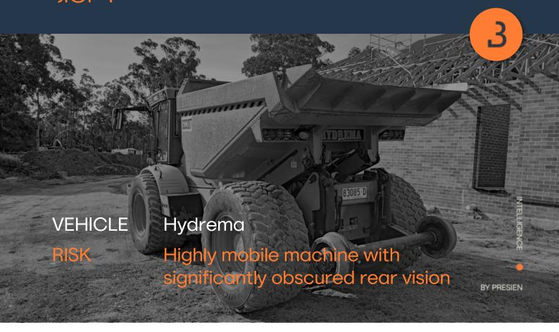
Operators and site health and safety were concerned of potential plant-people interaction at the truck's rear blind spot due to the quick and varied forwards and backwards operation of the vehicle.
