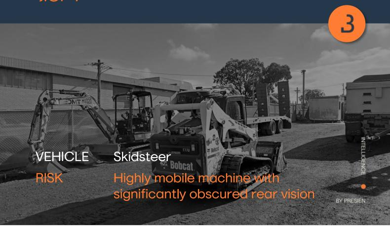
Operators and site health and safety were concerned of potential plant-people and plant-plant interaction at the skidsteer's rear blind spot, due to the quick and varied forwards and backwards operation of the vehicle.
