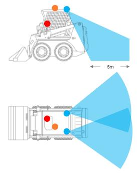
Hardware 1x Blindsight Processing Unit (BPU), 2x sensor with magnet mount, 2x 5m cable, 1x
