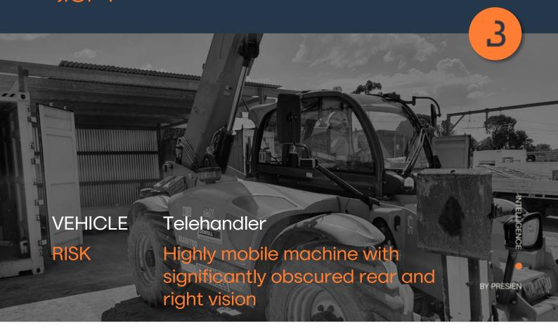
Operators and site health and safety were concerned about the telehandler's close quarter proximity to on-foot personnel. When loaded, the boom arm completely obscures the operator's vision on the right side, creating a dangerous potential for people-plant interaction.
