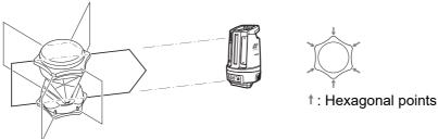
ATP2SII:The 360° Prism should be set up so that a pair of diametrically-opposed marks on top of the prism are aligned with the sighting direction of the instrument.
