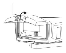
2. Check the orientation of the terminal of the battery, and then insert the battery by sliding it to the right and pressing against the main unit.
