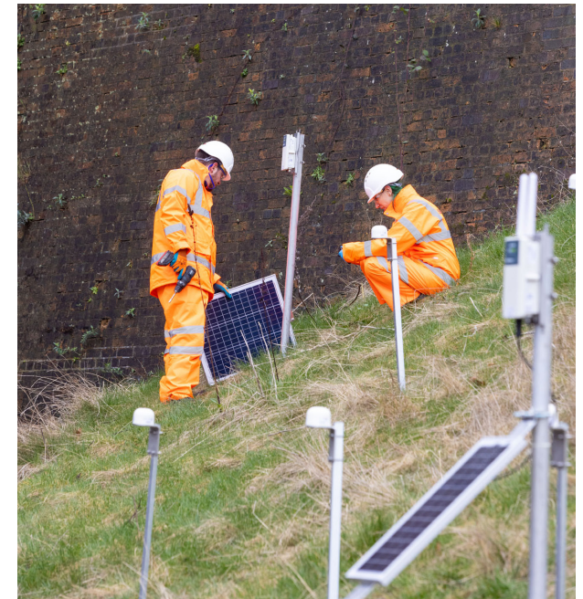
Picture 2: A typical InfraGuard™ deployment comprises rows of tilt sensing nodes fixed to metal stakes, together with a 4G Gateway, and a 4G camera
