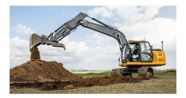
The Topcon MC-Max allows us to work 25 to 30% faster than using (versus) a conventional machine.
