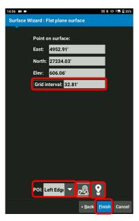
In order to create a new flat plane surface, define the reference height/coordinate for the flat plane surface
