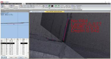
Comprehensive road defect / pothole detection and analysis tools. All defects are numbered by chainage and offset and analysed by area, depth and volume. Defects can be scrolled through in a combined section and plan view. Full output to CAD and reports with full analysis and supporting graphics.
