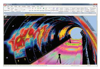
Un-roll and re-roll cylindrical and box tunnel models, and highlight and annotate design differences
