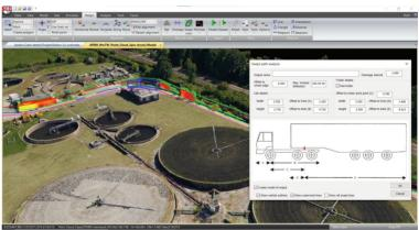
Vertical shaft and tank design with modelling and comparison to scanned point clouds. Support for unwrapping and rewrapping, with analysis and annotation of deviation between design and measured models. Support for both circular and template based designs across simple and complex alignments.
