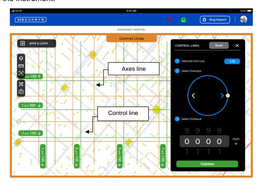
Figure 26 - Validation of a control line
