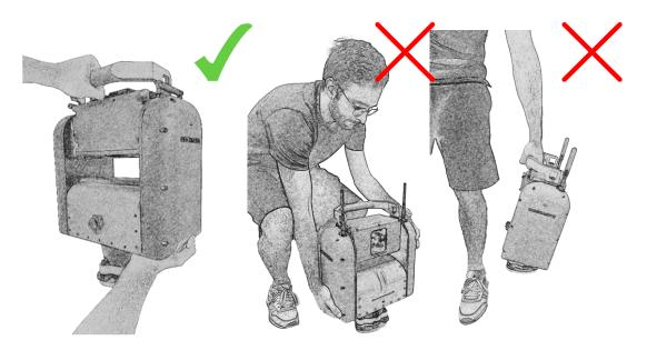
Figure 13 – How to carry the instrument
