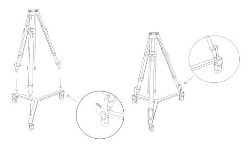
Figure 12 - Placement of the tripod on the wheel system
