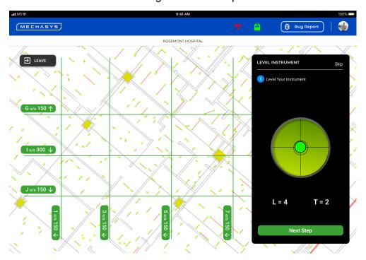
Figure 28 – Graphical interface of the digital level of the instrument
