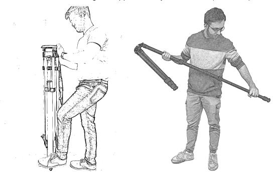
Figure 8 – Recommended Tripod Height
