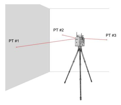
Figure 38 - Laser pointer positioning on walls
