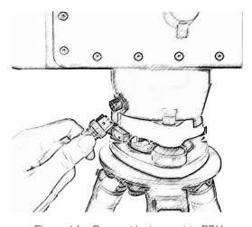
Figure 14 - Connect instrument to PSU
