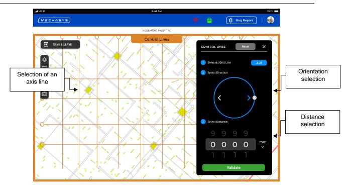
Figure 25 - Offset of a control line
