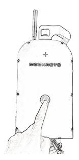
Figure 16 - Starting up the instrument
