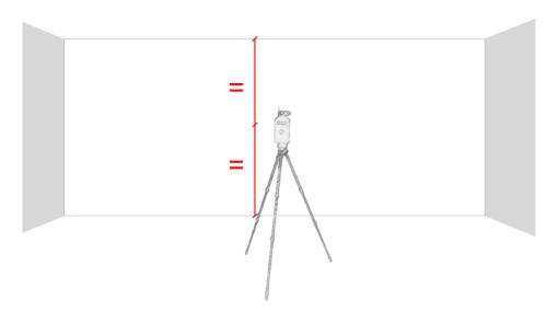
Figure 11 – Height for floor and ceiling projection
