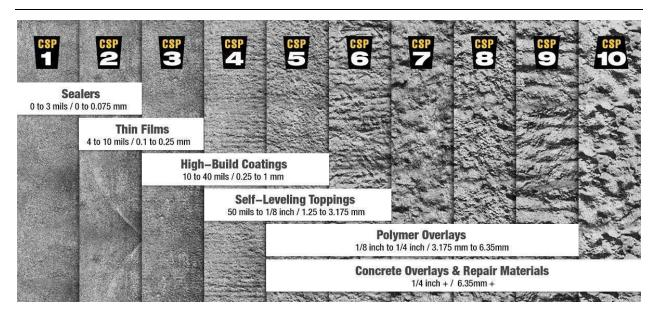
Figure 50 - Categorization of supported surfaces (source : graco.com)
