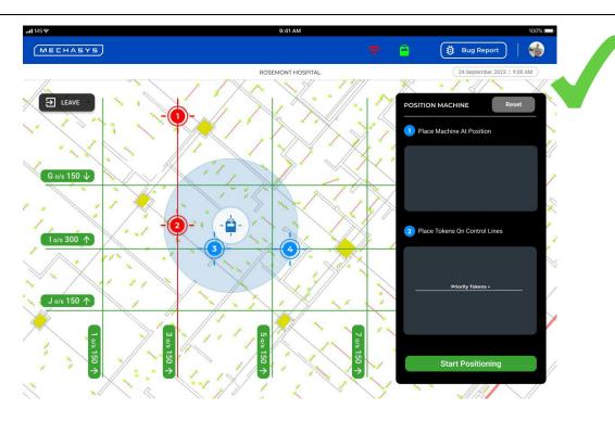
Figure 33 - Good positioning of the tokens on control lines
