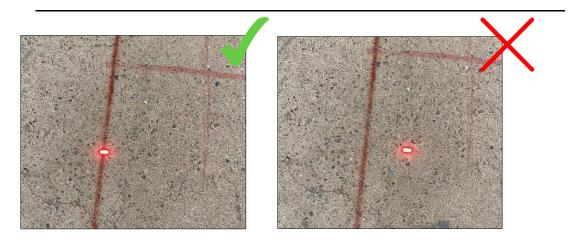
Figure 37 - Laser pointer positioning for control line
