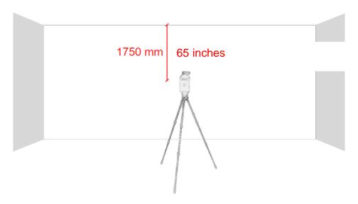
Figure 10 – Height from the ceiling
