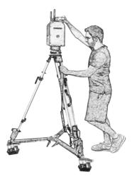
Figure 44 - Station to station transportation – Recommended technique with wheels
