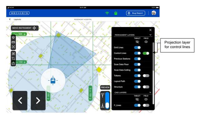
Figure 41 - Control lines layer
