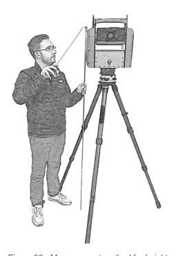
Figure 30 - Measurement method for height
